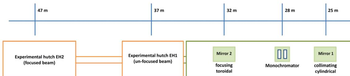
**Figure 1.** Sketch of the proposed beamline: the Optic Hutch (OH) contains all the main optical elements whereas the experiments are carried out in the Experimental Hutches EH2 (focused beam) and EH1 (unfocused beam). In the upper part of the picture the distance of the various elements from the source is indicated.
