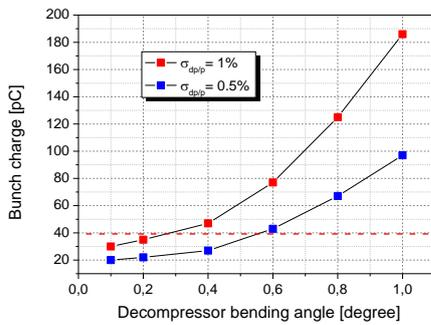
**Figure 4:** Require bunch charge to provide the peak current of 4kA for different bending angle of the decompressor dipole magnets in the case of different initial RMS energy spread  $\sigma_{\Delta p/p}=1\%$  or 0.5%.
