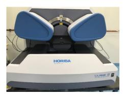
film. The ellipsometer allows the user to analyze the polarized light according to the reflection angle and the beam wavelength.
