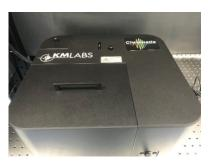
Chromatis dispersion instrument is another designed and built by KMLabs and capable to measure group delay dispersion in 1" and 2" optical components for femtosecond applications. The Hamamatsu Streak camera is an ultrahigh-speed detector which captures femtosecond light pulses.
